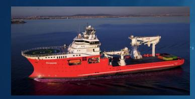
OFFSHORE CONSTRUCTION SUBSEA VESSEL, 130M X 25M, TRIPLE REDUNDANCY, 300 TONS SWL AHC OFFSHORE CRANE
