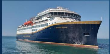
WORLD'S LARGEST BATTERY CAPACITY PASSENGER VESSEL 124 X 28M, 716 PERSON CAPACITY, 6500 KWH BATTERY
