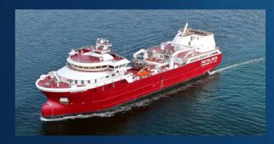
%100 LNG FUELLED LIVE FISH CARRIER 86 X 18 M, 4300 M3 CARGO HOLD CAPACITY, HAVFARM CONNECTION SYSTEM
